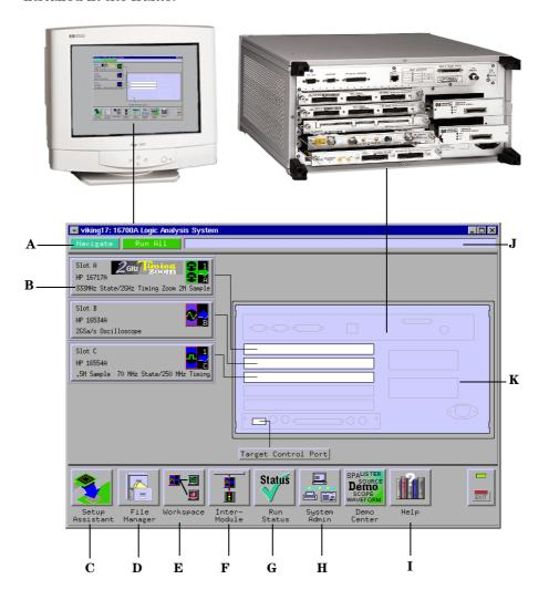
**A** *Navigate* is used to access instruments and the windows such as Setup..., Waveform..., Listing..., and the Source Viewer... window.
