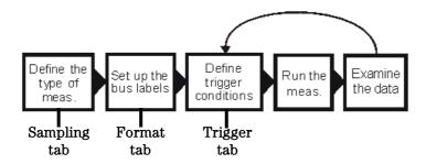
**Define the type of measurement.** Define how you want to sample data by selecting state mode or timing mode, and by setting up the state clock.
