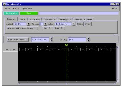
**4** To the right of the *Seconds/div* field click on the down arrow until the field is set to 50 ns. This will zoom in on the waveform.
