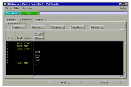
The "walking ones" program is complete. The pattern generator will output 0001, 0010, 0100, 1000 to the logic analyzer.
