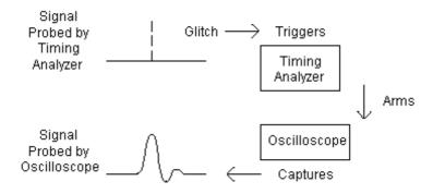
In this chapter, you will capture the glitch on the credit card board by using the timing analyzer to trigger the oscilloscope. This chapter steps you through setting up the timing analyzer and bus labels, triggering on the glitch, making an intermodule measurement, and importing the analog waveform into the timing waveform window.
