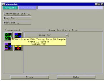
**4** When you find the analyzer you are using, click on it and hold the mouse button down to select *Group Run*.
