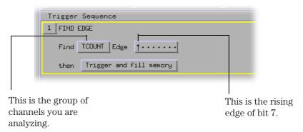
You have finished setting up the analyzer to trigger on the rising edge of bit 7. You are now ready to run the analyzer and capture data.
