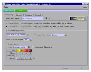
Each pod has one clock channel. The clock channel on pod 1 is J. We will set J to sample data on the falling edge.
