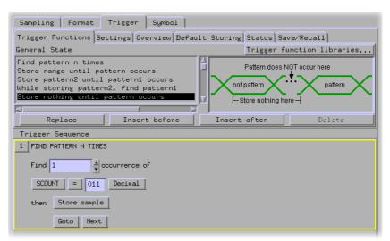
To tell the analyzer to find the rest of the sequence 022, 033, and 044 before triggering, we will set up three more sequence levels similar to the one finding 011.
