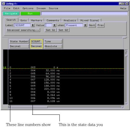
These line numbers show the locations of the data in the logic analyzers memory. This is the state data you captured from the credit card board.
